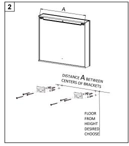
2. Screw the bracket to the wall by using the screws provided.
