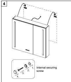
3. Hang the cabinet on the wall bracket, the claws on the cabinet hangers must be securely located on the wall bracket.(the position of cabinet can be adjusted about 10cm for left side or right side)
